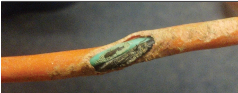
Figure 2: An electrocution incident and layout of the breeding and gestation barn where the incident occurred are described in Figure 1. The damaged area of the 100-foot extension cord is shown. This type of damage suggested that rodents had chewed the cord's outer insulation, allowing the flow of current through the metal of the pens and stalls.
